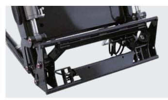
Implement locking mechanism at the touch of a button, making it even more convenient to change the implement without having to get out of the cab – with HYDRO-LOCK.
