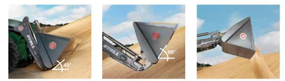
This is what it looks like in action: A full bucket remains full even when it is being lifted, thanks to the rescooping function. The result: No trickle losses, high loading capacity. The system is as simple as it is ingenious. After the bucket has been lifted, it can be tilted 24° again while the loader is lifting. This keeps the load in the bucket.
